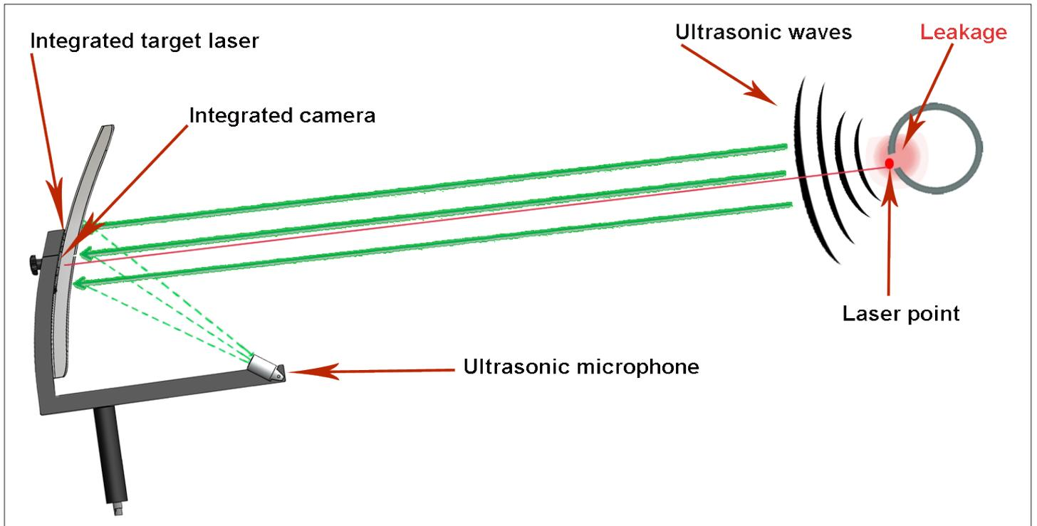
By bundling the ultrasonic waves in the parabolic mirror, even the smallest leaks of 0.8 l / min (ca. 8 € p.a.) at a distance of up to 10 ... 15 m can be localized with pinpoint accuracy ( $\pm 15$  cm). The shape of the parabolic mirror ensures that only ultrasonic waves of the targeted leak are evaluated. Disterbing noise is reduced to a minimum.
