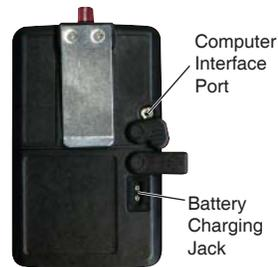
**!** *Ensure proper orientation of charging cable before plugging it into the charging jack. Improper orientation/contact will short-circuit the battery. See photo at right. Note the keyed side of the charging cable plug must mate with the keyed side of the pump charging jack. Inserting the plug does not take much force. If force is required, the plug is not properly oriented.*
